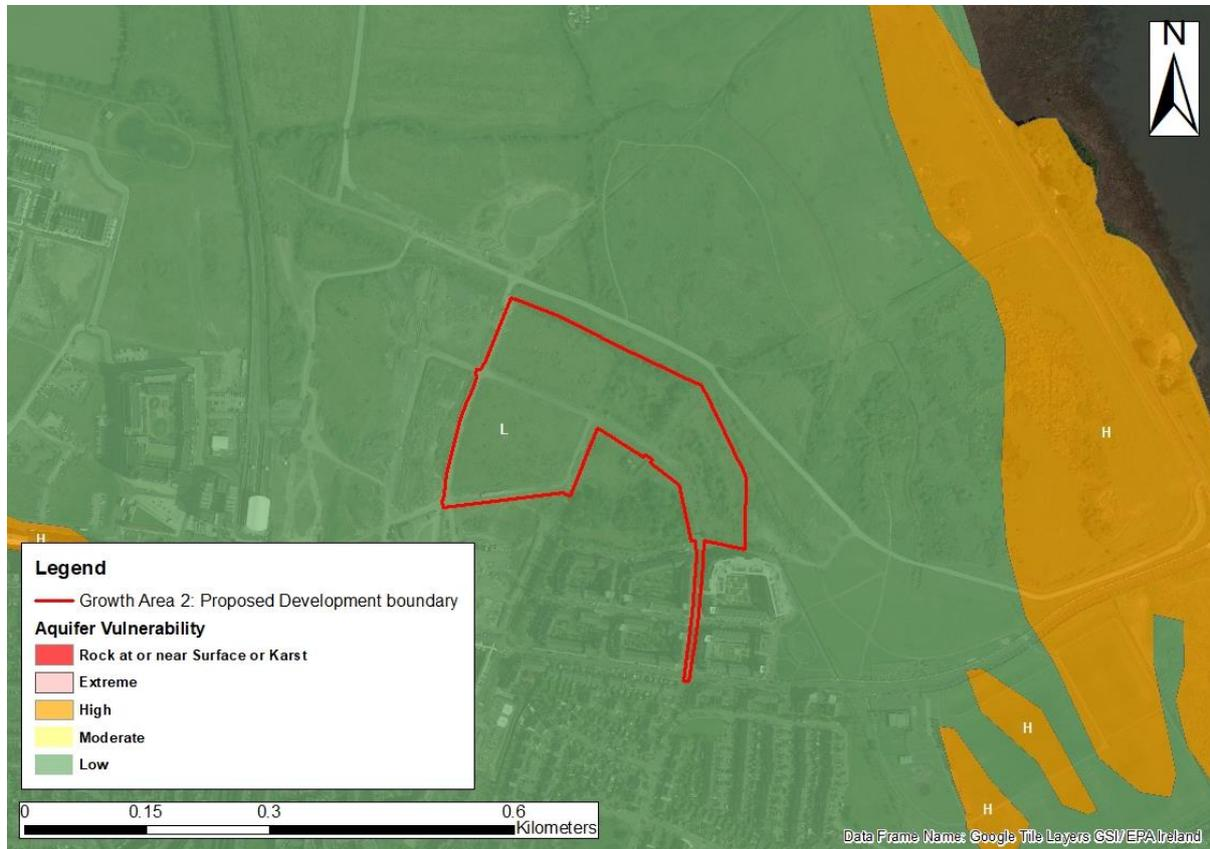
**Figure 7.3.2** Aquifer Vulnerability Map with the proposed site layout (Source: GSI, 2022)
