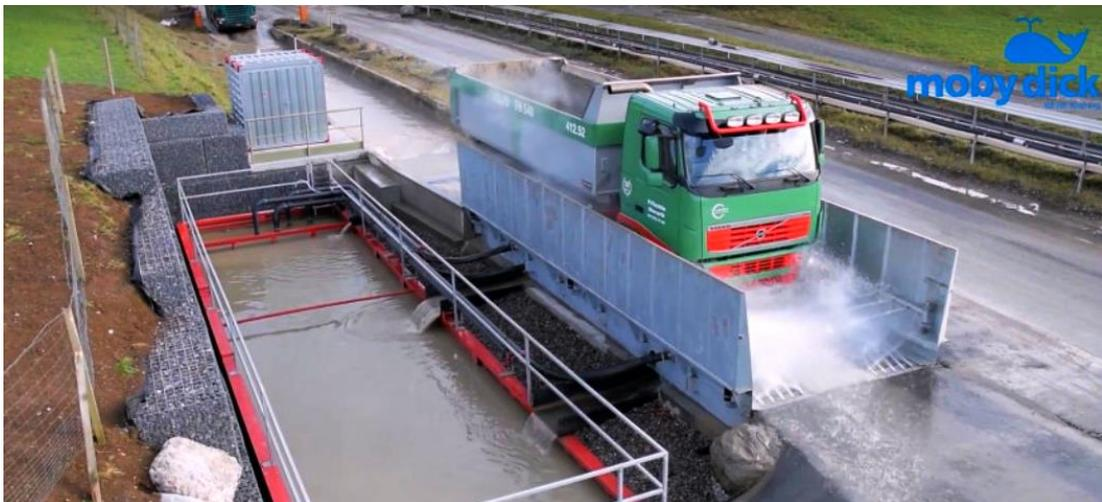
Figure 5.1 Example of Wheel Washing System
